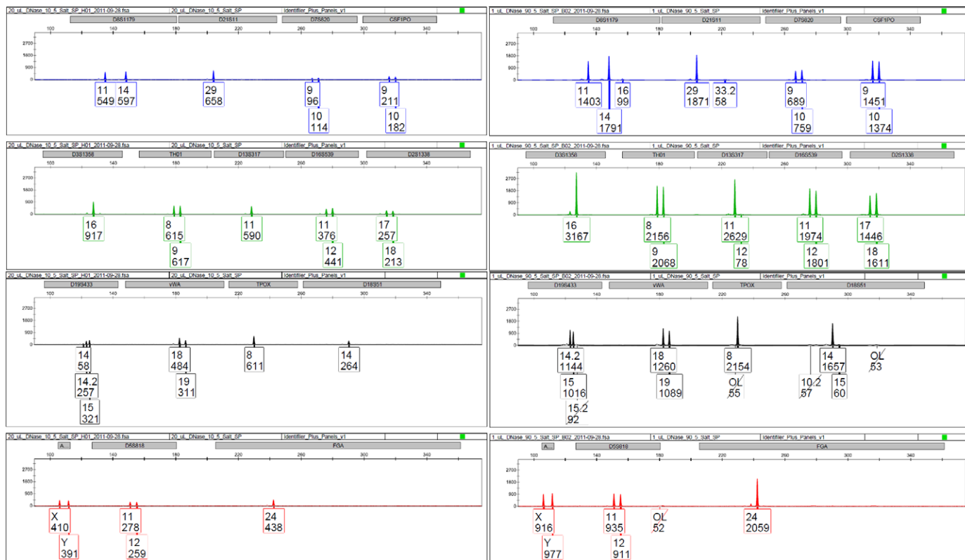
FIG. 4—Electropherograms of duplicate samples digested with varying amounts of DNase. Data scaled to 3500 RFUS. The profile on the left was prepared with the initial Garvin et al. recommended DNase and ionic concentration, resulting in very low peak heights. The profile on the right was prepared with the optimal DNase and ionic concentration, showing significant improvement in peak height. Trace alleles consistent with carryover from the nonsperm fraction were observed in the profile on the right. This is a result of the DNase not being 100% efficient in removing all residual amounts of nonsperm DNA. See sections below for further discussion.
